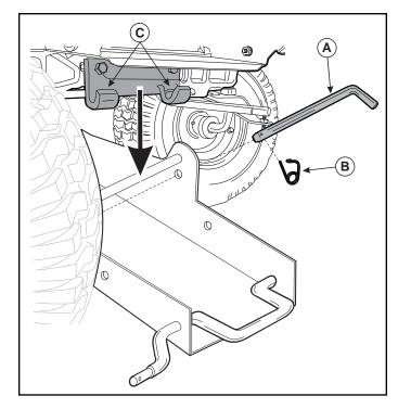
Figure 19. Remove Hitch Latch Pin
